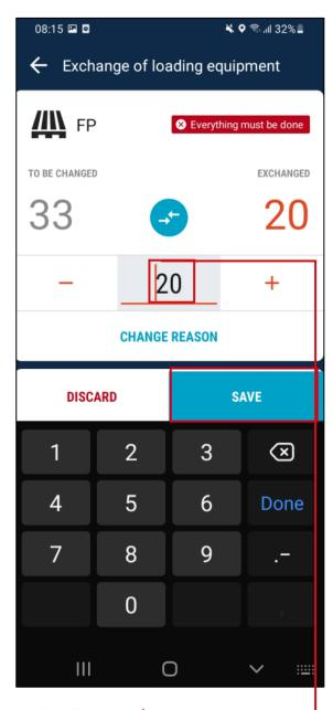
If there is no smooth exchange of loading equipment, first enter the number (in this case 20) that could be exchanged without problems and confirm this with "Save".
